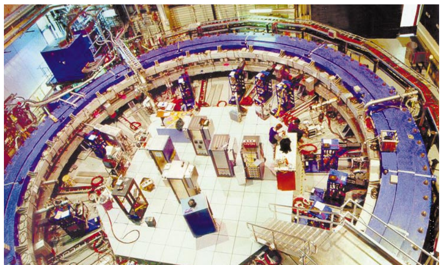
Figure 1 The 14-metre-diameter superconducting magnet used by the E821 experiment at Brookhaven National Laboratory, Long Island, New York. It provides a magnetic field of extremely high quality, allowing physicists to measure the magnetic behaviour of the muon with unprecedented accuracy.
